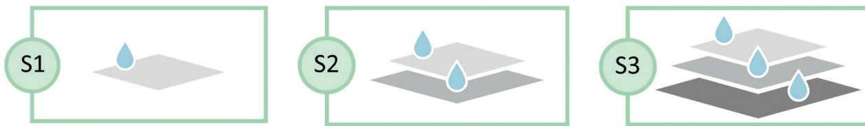
Figure 5: The BIM Barrier Standard helps us identify which properties are required. To meet the requirements up to three different barriers can then be applied in up to three layers.
